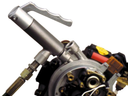
TW17H | Testing of injection pumps
